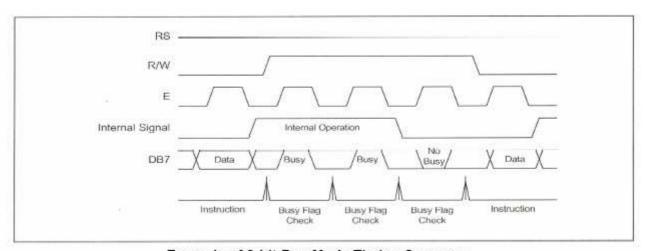
Example of 8-bit Bus Mode Timing Sequence
