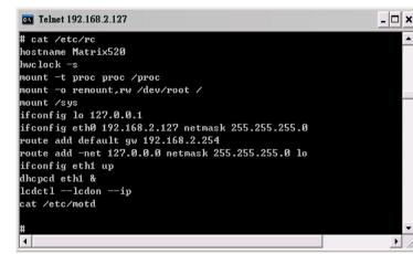
To configure the IP address, Netmask and Gateway setting, please modify /disk/etc/rc as following: *ifconfig eth0 192.168.2.127 netmask 255.255.255.0*
