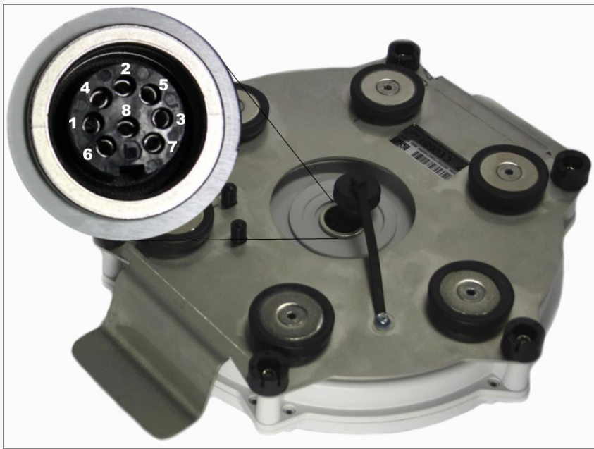
Figure 3: Pin assignments of the 6/8pin female socket.
