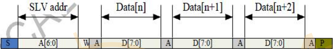
Figure 2-5 I2C master write, slave read
