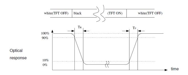
Note (4) Definition of optical measurement setup
