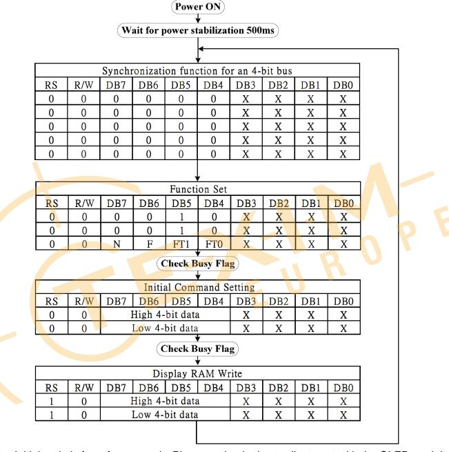
Note: Initial code is for reference only. Please make the best adjustment with the OLED module.
