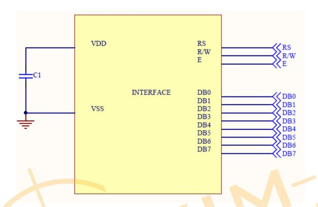
Pin connected to MCU interface: RS, R/W, E, DB0~DB7
