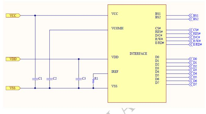
Recommended components: C1, C2 : 2.2uF/25V/0603 C3 : 1.0uF/16V/0603
