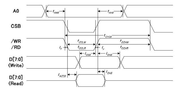
\*1 The input signal rise time and fall time (tr, tf) is specified at 15 ns or less. When the system cycle time is extremely fast,
