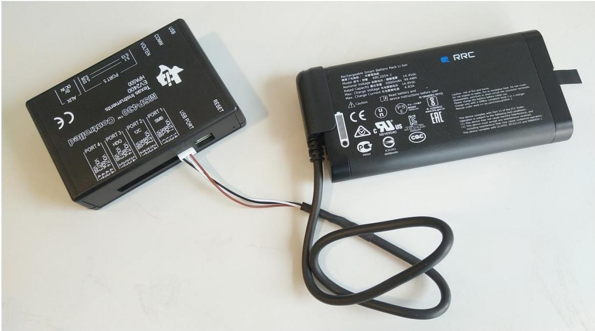
3. Then connect EV2400 (USB Type B) to PC with USB-cable (part of EV2400 evaluation kit):
