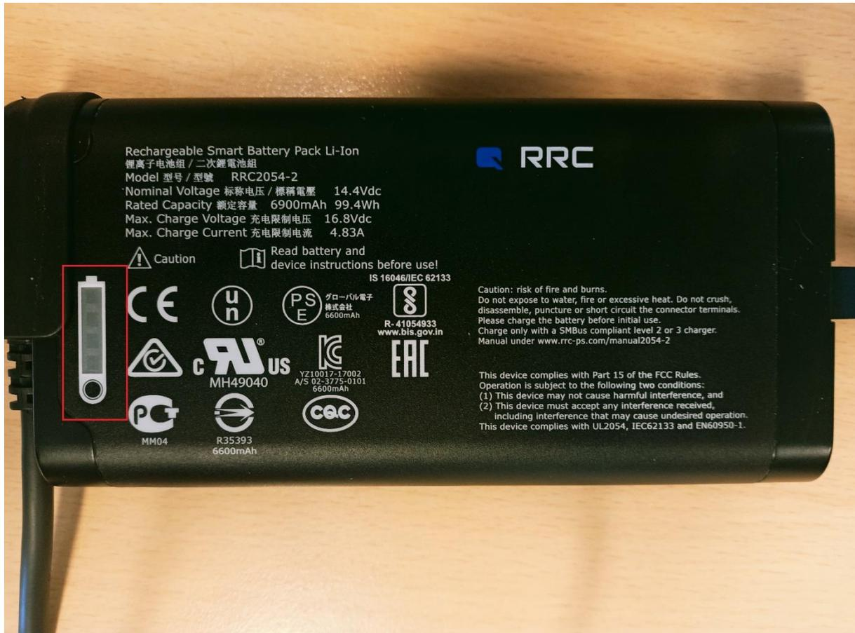
When pressing on indicator button, and battery is not in shipping mode, one or more green LEDs are active depending on status of charge. If no LED is active the battery can be in shipping mode or empty.
