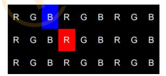
**Three or more adjacent dots (horizontal):** Use the bright spot illustration as an example to demonstrate three or more consecutive horizontal and vertical dots.
