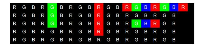
**Illustration of spacing between two dots:** (Distance is the relative distance between the X-axes of the two dots or the relative distance between the Y-axes of the two dots, whichever is larger)
