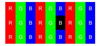
Two adjacent dots (horizontal direction): Use the bright dot illustration as an example to demonstrate two horizontal consecutive dots.
