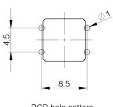
PCB hole pattern component side
