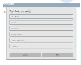
To help to configure or install the MODBUS product, a function to test writing into the register of a slave has been integrated into the advanced mode of the IoT Configurator.
