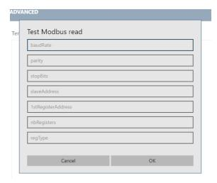
To help to configure or install the MODBUS product, a function to test the reading of a slave has been integrated into the advanced mode of the IoT Configurator.
