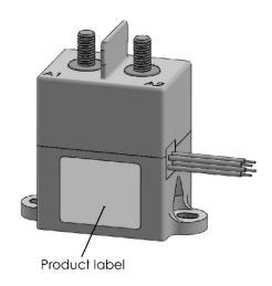
load input terminals - no polarity
