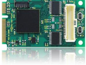
from the card. The digital I/O is compatible with 8255 PPI chips making it easy to program. This allows for simple and trouble-free migration from other ACCES PCI and PCI Express digital I/O cards, but also provides for advanced features enabled by the onboard FPGA logic.
