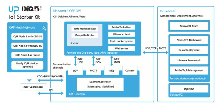
UP board is connected to the IQRF network via SPI interface (adapter) of via CDC interface (GW-USB/CK-USB).
