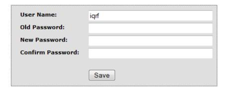
Both User name and the Password are default preset to "iqrf" from the factory. The password should be changed by the user on the *Password Setup* page. To accomplish the change, the original password and the new one must be entered. For security, the new password must be typed two times.
