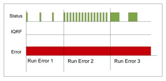
During run error red LED is continuously on. Green LED flashes with the specific duty:
