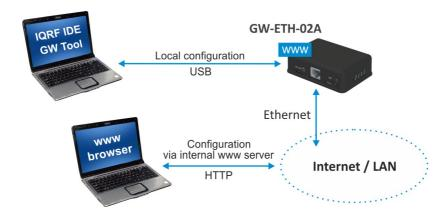
GW configuration is possible via internal www server, IQRF IDE or (especially for troubleshooting) via SD card.
