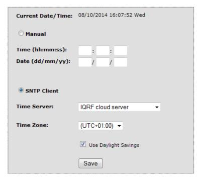
The *Time Setup* allows to set the time of the internal clock measured by the GW. The time is required especially for the datalogger. Individual logs are provided with time stamps. The time can be setup manually or via the SNTP service. The SNTP provides periodical time synchronization from one of selected time servers. As a time server, the IQRF Cloud server can be used as well. In the factory settings the time and date are synchronized with the IQRF Cloud server.
