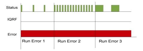
During run error red LED is continuously on. Green LED flashes with the specific duty:
