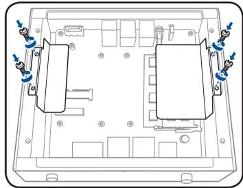
7. Secure the bottom cover to Nano-001 with the screws you removed earlier.
