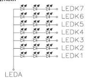
Note2:The LED of B/L is drive by current only, drive Voltage is for reference only, drive voltage can make driving current under safety area ( current Between minimum and maximum).50K hours is only an estimate for reference.
