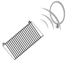
Copper wire that is part of the antenna is not isolated, therefore in order to avoid antenna short circuit, it is advisable not to place this bare tag directly on a metal surface. Placing a thin layer of non-conductive material between tag and metal is recommended or use our *FXTO.2-SLI-R* (protected with thermo-shrink rubber).
