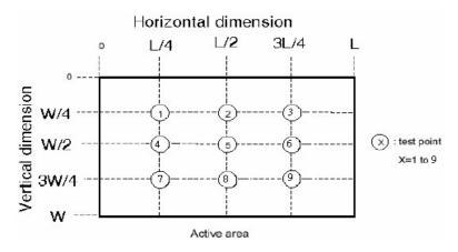
$$\left(\begin{array}{c} \text{MAX Luminance - Average Luminance} \\ \text{Average Luminance} \end{array}\right) \quad x100\% \quad \geqq 70\%$$
