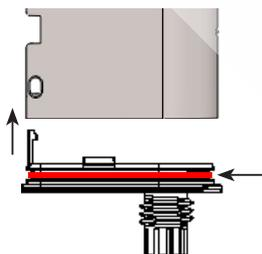
When you close the casing and in order to conserve the IP67 protection, be sure that the seal is not twisted or that the soleplate is correctly clipped.
