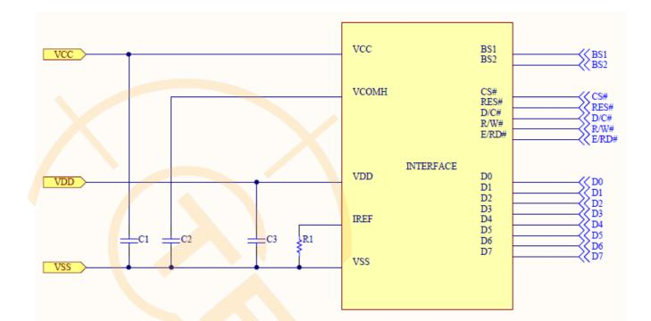
Recommended components: C1, C2 : 2.2uF/25V/0603 C3 : 1.0uF/16V/0603
