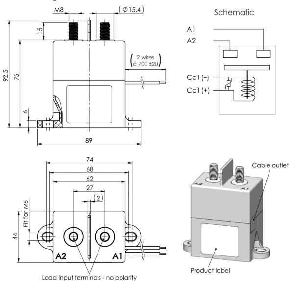
In case of no tolerance shown in dimensional drawing, general tolerances apply: dimension  $\leq 10$  mm;  $\pm 0.3$  mm; dimension 10 to 50 mm; dimension > 50 mm;  $\pm 1$  mm
