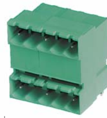
pitch 10/10.16 mm from 1 to 13 poles 90° version, polarized
