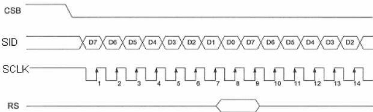
Note: Following is the master SPI clock mode of MPU.
