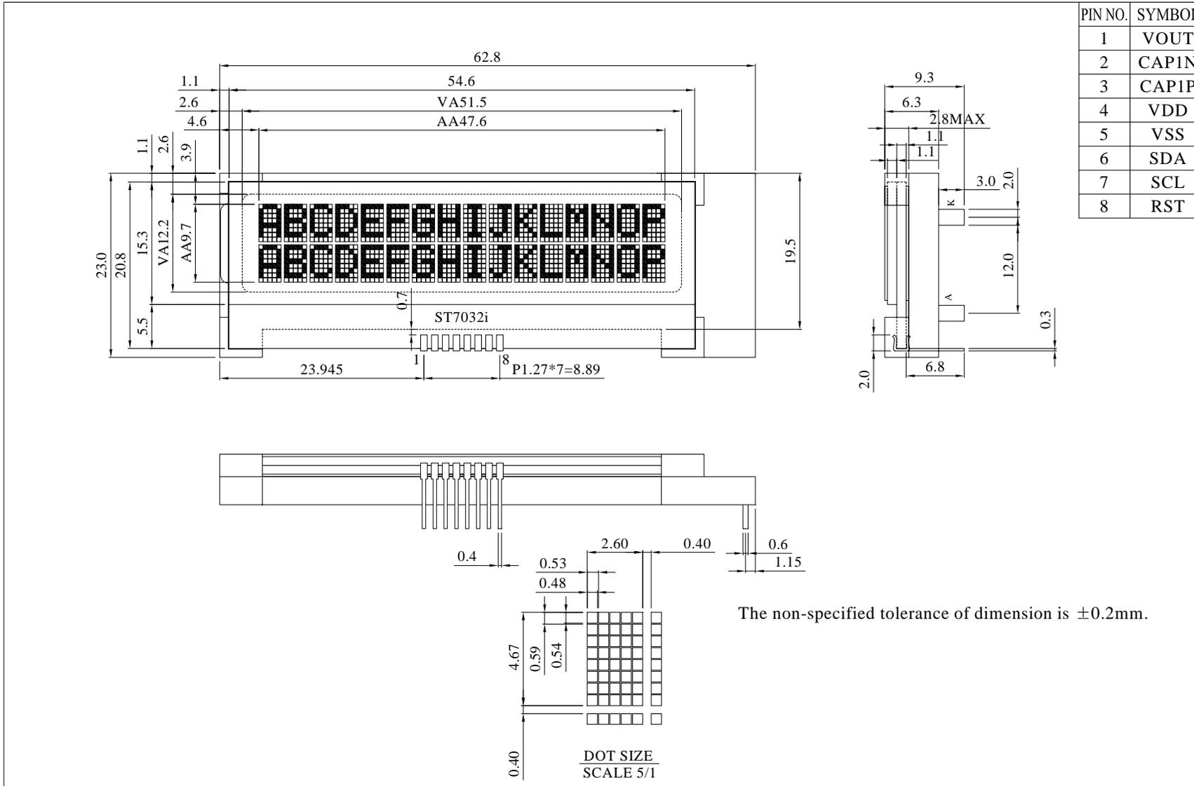
The non-specified tolerance of dimension is  $\pm 0.2\text{mm}$ .
