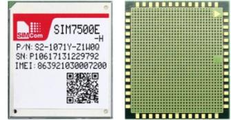
The SIM7500E-H is Multi-Band LTE-FDD/WCDMA/GSM module solution in a LGA type which supports LTE CAT4 up to 150Mbps for downlink data transfer.
