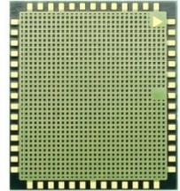
The SIM7500E is Multi-Band LTE-FDD/WCDMA/GSM module solution in a LGA type which supports LTE CAT1 up to 10Mbps for downlink data transfer.
