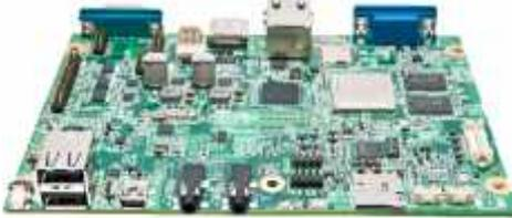
BF8A1 is a 3.5" compact board with an on-board Freescale i.MX6 solo, dual or quad cores 1.0GHz CPU with up to 2GB RAM and 4GB eMMC onboard. This 3.5" SBC features several video output ports (HDMI, VGA, LVDS 24-bit interface), one Gigabit Ethernet, four USB ports and four COM ports and one mini PCI Express slot for additional expansion.
